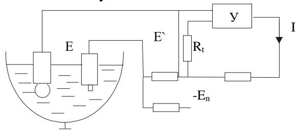
$$E' = E - E_\Pi = 0,059(pH - pH_\Pi)[1 + \alpha(t - t_0)] = U_{\text{вых}}$$
